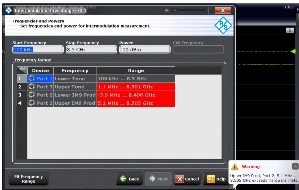
Figure 8 - Frequency range: Defining and viewing exceeded limits
