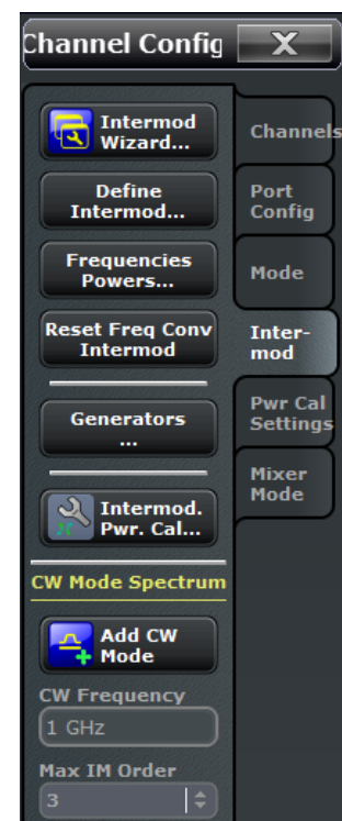
Figure 27 - Editing the intermodulation measurement configuration
