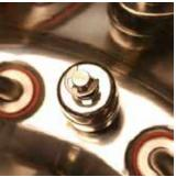
Low water sensor prevents damage by sounding an alarm and stopping all operations until water is refilled
