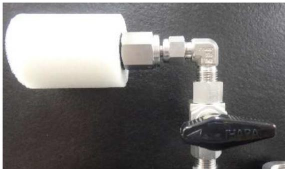
The gas ballast mechanism prevents condensable gases (such as water vapor and solvent-laden gases) from condensing inside the pump, thereby extending the pump's lifespan.
