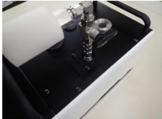
The gas ballast mechanism is not installed in the pump upon delivery. Installation instructions can be found in the operational manual provided with the unit.
