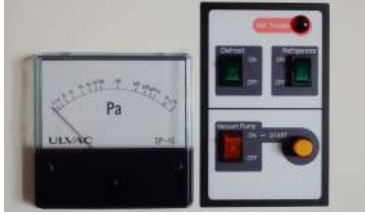
Pirani Vacuum Gauge and Control Panel
