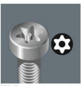
TORX® tools with a borehole unauthorised prevent the unfastening of safety screws. The screws contain a pin that protrudes into the drive profile so that "normal" TORX® tools cannot be used. This pin fits into the borehole of TORX® BO tools allowing safety screws to be unfastened.
