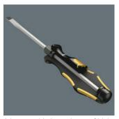
A hexagon blade made out of highquality bit material extends right through the handle - thereby ensuring full transfer of force, even when struck with a hammer. The ductile tempered material prevents the blade from splintering or breaking.
