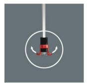
The two gripper arms spread further apart as they are pushed surface against the and automatically snap back when the head of the screw is countersunk.
