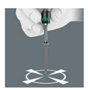
The free-turning sleeve allows screw steadying at the start of the screwdriving process. This makes it easier to apply the tool to the screw and prevents slipping. It can also be used as a short extension for 1/4" applications e.g. in combination with the Wera Zyklop Ratchets.
