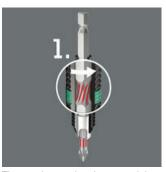
The torsion spring integrated into unique BiTorsion holder the absorbs lower levels of peak loads (Phase 1). Any overloading of this spring is effectively prevented by means of а supporting mechanism.
