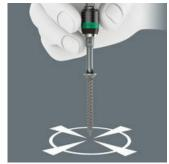
The free-turning sleeve allows screw steadying at the start of the screwdriving process. This makes it easier to apply the tool to the screw and prevents slipping. It can also be used as a short extension for 1/4" applications e.g. in combination with the Wera Zyklop Ratchets.
