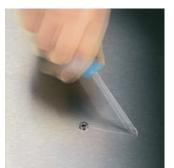
It happens time and time again that the tip slips out of the screw head when screwdriving, sometimes damaging valuable surfaces or even causing injury. The tips of the Wera Lasertip screwdrivers are microscopically roughened by means of a laser. This rough surface literally "bites" itself firmly into the screw head. Slipping out becomes a thing of the past.
