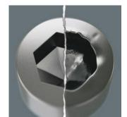
Hexagon screws can endure a problem because the contact surfaces delivering the power from conventional the tool, is transferred to the screw via very small surface areas. The consequence: the screw can become damaged (rounding out). Hex-Plus tools have a greater contact surface that prevents this from happening! At the same time, as much as 20 % more torque can be applied. Good to know: Hex-Plus tools fit into every standard hexagon socket screw!
