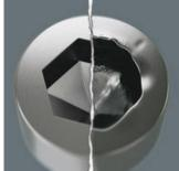
Hexagon screws can endure a problem because the contact surfaces delivering the power from conventional tool, is transferred to the screw via very small surface areas. The consequence: the screw can become damaged (rounding out). Hex-Plus tools have a greater contact surface that prevents this from happening! At the same time, as much as 20 % more torque can be applied. Good to know: Hex-Plus tools fit into every standard hexagon socket screw!
