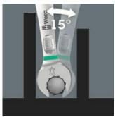
The Joker 6003 ring spanner with its special mouth geometry mouth side pivoted by 7.5° and the double hexagon profile doubles the placement possibilities when repeatedly turning wrench 180° around the longitudinal axis. Bolts and screw heads can be "accessed" every 15°. The Joker 6003 will automatically find the respective placement point after every turn.
