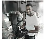
The compact folding pouch with adjustable Joker 6004 spanners covers all metric and imperial dimensions in applications from 7 to 19 mm or 1/4" to 3/4"
