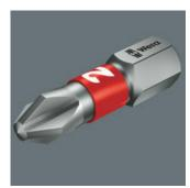
BiTorsion bits are absolutely premium products. They have a BiTorsion zone which reduces the hardness of the shaft by about 20 % in comparison to the drive tip. This means that the peak loads that cause bit breakage and premature wear are absorbed in this zone - something which enhances the service life of the bits.
