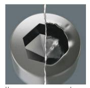
Hexagon screws can endure a problem because the contact surfaces delivering the power from the conventional tool, is transferred to the screw via very small surface areas. The consequence: the screw can become damaged (rounding out). Hex-Plus tools have a greater contact surface that prevents this from happening! At the same time, as much as 20 % more torque can be applied. Good to know: Hex-Plus tools fit into every standard
