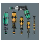
Wera torque screwdrivers. With a factory pre-set torque value set to the smallest scale value. For all applications, where the same constant torque and repeat accuracy are required. The torque can be changed with an extra tool within the measuring range (recalibration kit can be ordered with the code number 05137001001). Afterwards you can check the set value using an off-the-shelf torque tester.
