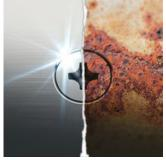
Stainless steel has the property of not rusting. However, if tools made out of conventional steel are used for stainless steel components or screws, the particles left behind from these tools can adhere to the surface and then rust. This effect known as extraneous rust - can impair the visual appearance and even cause structural damage that may result in expensive repair work. The wear particles that cause this rust effect can be prevented by using stainless steel tools.
