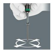
The free-turning sleeve allows screw steadying at the start of the screwdriving process. This makes it easier to apply the tool to the screw and prevents slipping. It can also be used as a short extension for ¼" applications e.g. in combination with the Wera Zyklop Ratchets.
