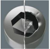
Hexagon screws can endure a problem because the contact surfaces delivering the power from conventional tool, transferred to the screw via very small surface areas. The consequence: the screw become damaged (rounding out). Hex-Plus tools have a greater contact surface that prevents this from happening! At the same time, as much as 20 % more torque can be applied. Good to know: Hex-Plus tools fit into every standard hexagon socket screw!
