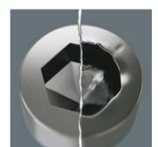
Hexagon screws can endure a problem because the contact surfaces delivering the power from conventional the tool, is transferred to the screw via very small surface areas. The consequence: the screw can become damaged (rounding out). Hex-Plus tools have a greater contact surface that prevents this from happening! At the same time, as much as 20 % more torque can be applied. Good to know: Hex-Plus tools fit into every standard hexagon socket screw!
