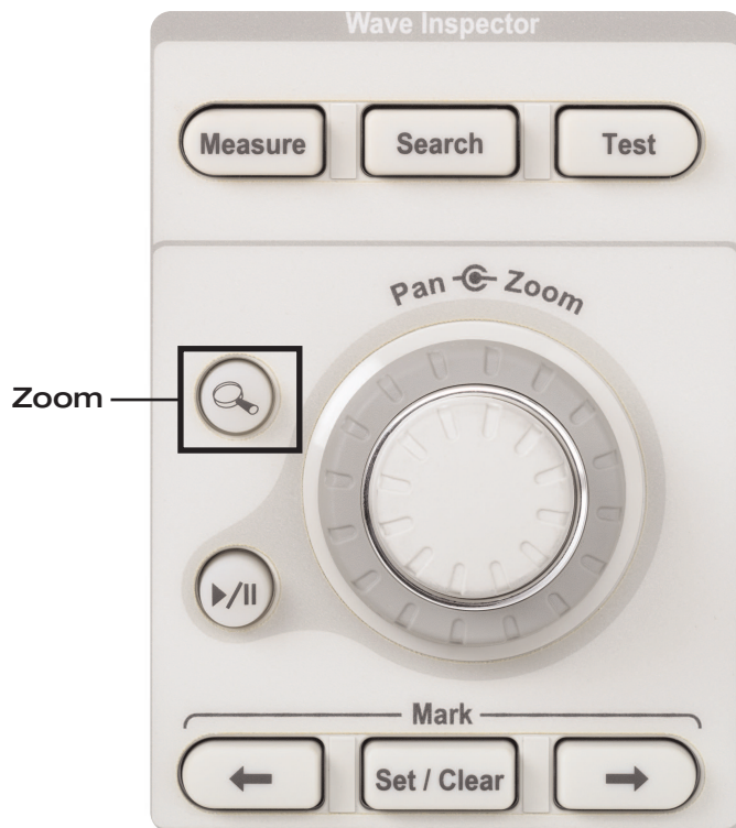
► Figure 1A. Wave Inspector® provides dedicated front panel zoom and pan controls.
