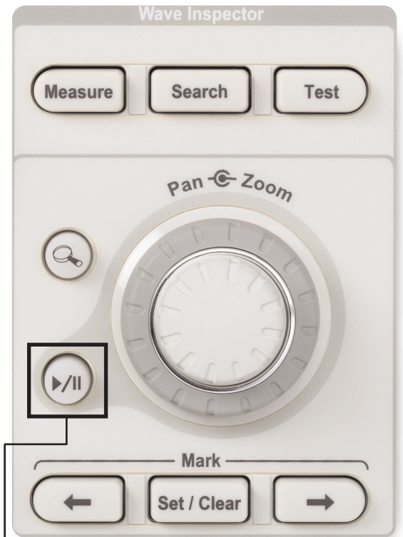
► Figure 2A. Dedicated front panel control for automated waveform playback.
