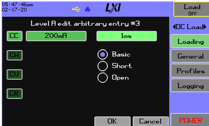
Figure 5-19 Level A Edit Arbitrary Entry #3
