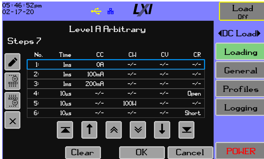
Figure 5-18 Level A Arbitrary Screen
