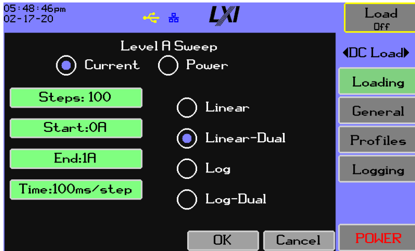
Figure 5-20 Level A Sweep Screen
