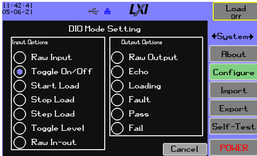
Figure 5-50 DIO Mode Setting
