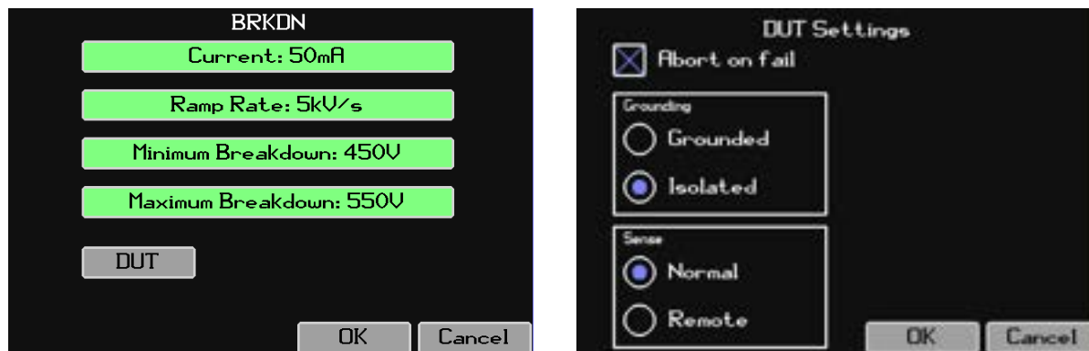
Figure 7-25 BRKDN Step Configuration Screens
