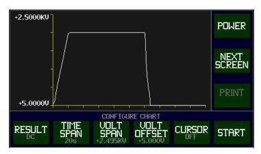
The 4700 can collect DC and AC measurement results over a user configurable time span. Starting data collection can be performed either manually or automatically. The measurement results are configured on the Primary Measurement Results Screen.
