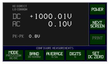
The main section of this screen shows the selected input terminals to the 4700 and the measurement results. If an input is in overload then the overloaded input terminal name is shown in red, and also the measurement results are shown in red.
