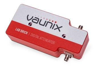
The Lab Brick LDA series of Digital Attenuators bring affordability, functionality, reliability, and simplicity to the microwave test bench. The LDA products range from 10 MHz to 40 GHz with input level tolerance to 2 Watts and step size as small as 0.1 dB.
