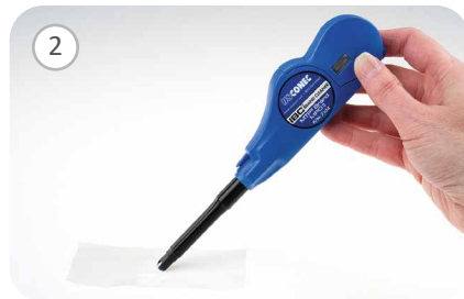
2 Lightly touch the cleaning ribbon/thread to the wet area of the wipe. Do not soak the ribbon/thread. Excessive cleaning solvent will require additional dry cleans
