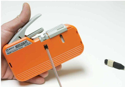
Placing PRIZM® LightTurn® connector into cleaner
