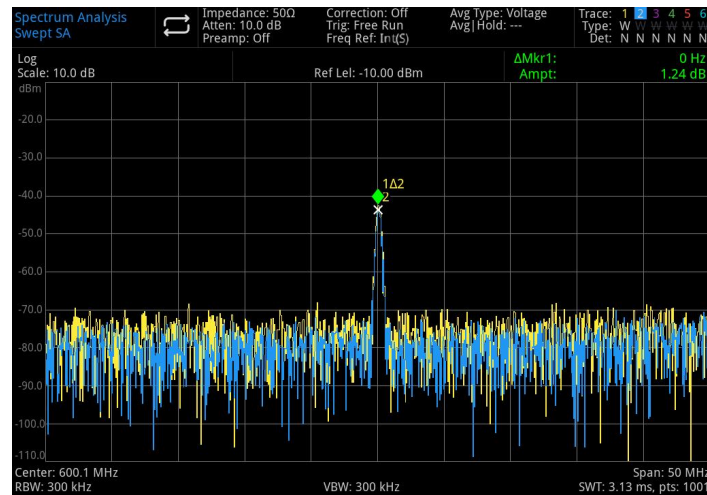
Figure 3-17 Component of Harmonic Distortion
