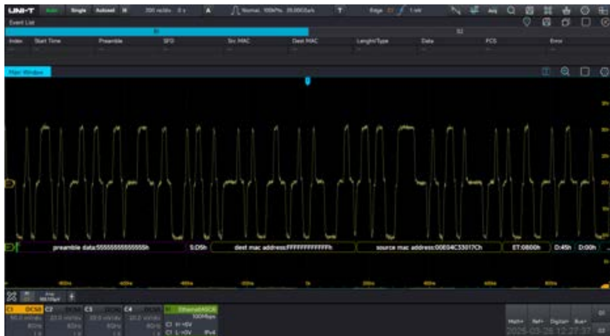
Analyze the 100M Ethernet bus. The bus waveform provides time-related decoded packet content, including preamble data, start frame delimiter, destination media access control address, source address, etc. The event list displays all the collected packet content.
