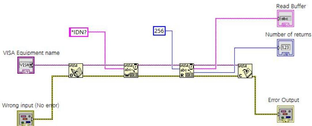
5. Communication with the device via TCP/IP is similar to USBTMC. You need Set the VISA Write and Read functions to synchronous I/O, as LabVIEW uses asynchronous I/O by default. Right-click on the node and select “Synchronous I/O Mode >> Synchronous” from the shortcut menu to enable synchronous writing or reading of data, as shown in the following figure.
