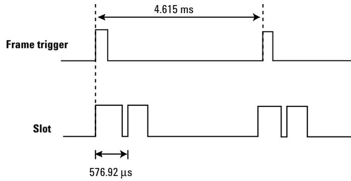
**Figure 6. Timing diagram of a GSM/EDGE signal**
