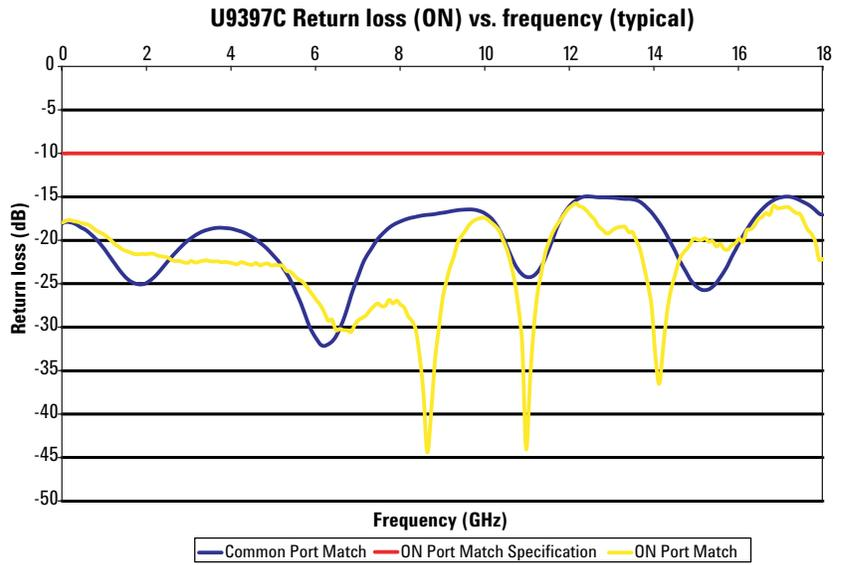
Figure 13. U9397C return loss (ON) vs. frequency (typical)
