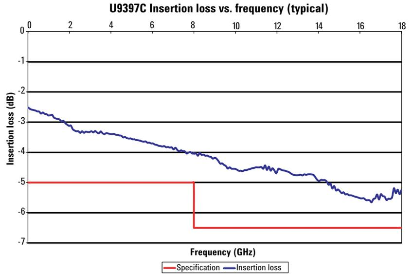
Figure 12. U9397C insertion loss vs. frequency (typical)
