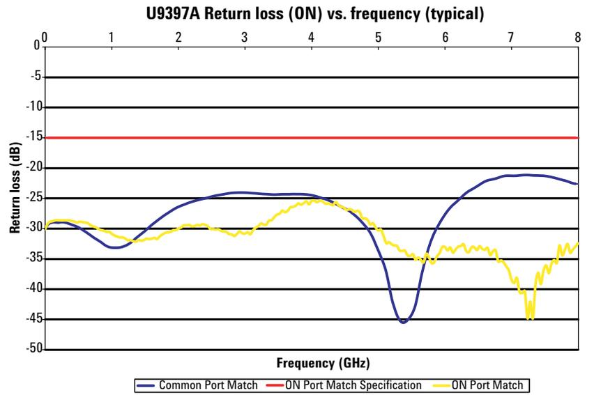
Figure 9. U9397A Return loss (ON) vs. frequency (typical)
