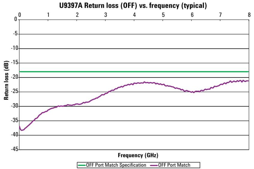
Figure 10. U9397A Return loss (OFF) vs. frequency (typical)
