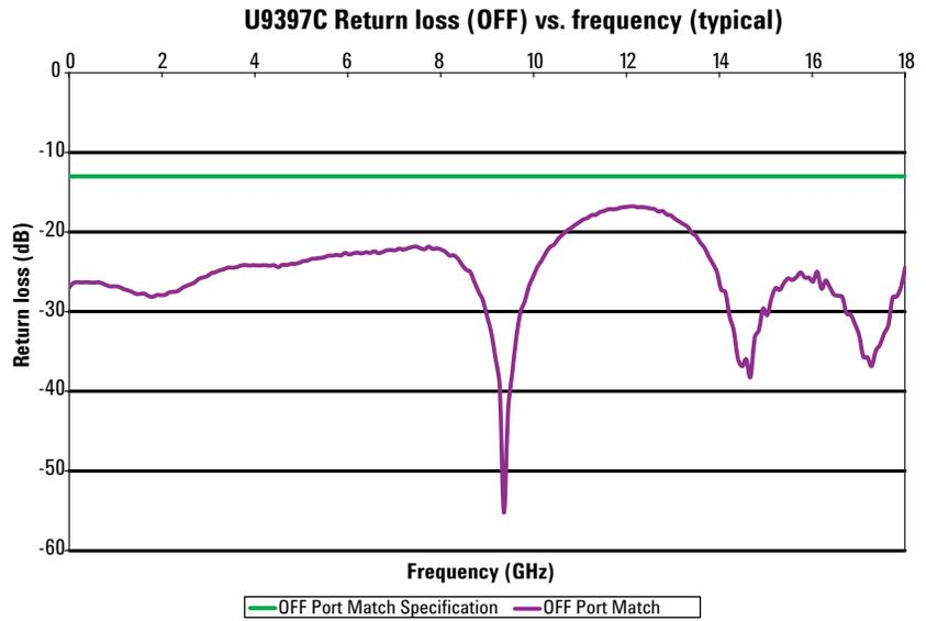
Figure 14. U9397C return loss (OFF) vs. frequency (typical)
