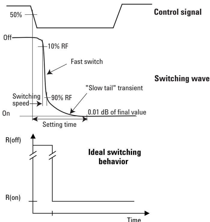
Figure 1. Comparison of ideal and real switching behavior
