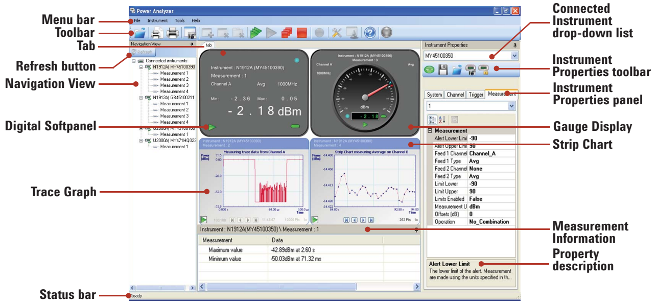
Figure 11: Advanced version of N1918A Power Analysis Manager, Power Analyzer
