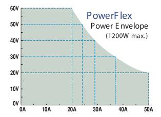
The QPX1200S is a laboratory dc power supply with a maximum total output power of 1200 watts and is suited to both bench-top and system applications. The QPX1200SP adds full digital remote control using USB, RS-232, LAN and GPIB interfaces. Both models include analog remote control.
