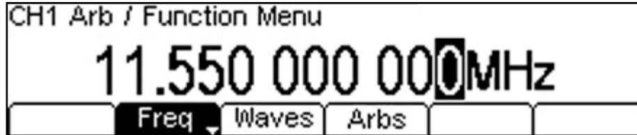
The lower frequency limit is 1mHz. The upper frequency limits is 50MHz [25MHz].
