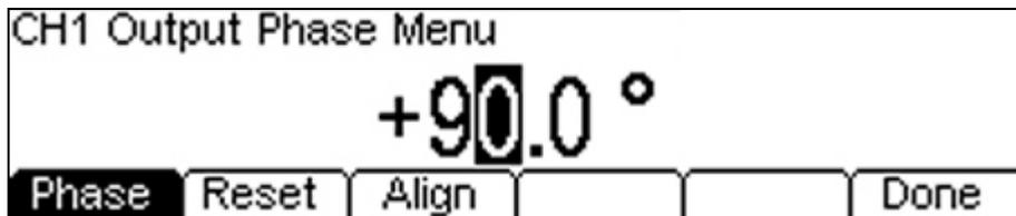
The current phase value is retained when the waveform type is changed. The **Reset** soft-key returns the phase to zero (0.0 degrees).
