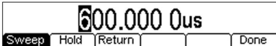
The **Sweep** time defines the time taken to go from the start frequency to the stop frequency.
