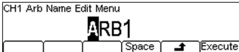
The name can be changed if required. A name of up to 8 characters can be used. The cursor keys < > are used to select the character and the spin wheel used to change the character. When the wheel is turned clockwise the characters change in the following order: 0 to 9, A to Z, ^ \_ ' { } ~ (space) ! # \$ % & ' ( ) -
