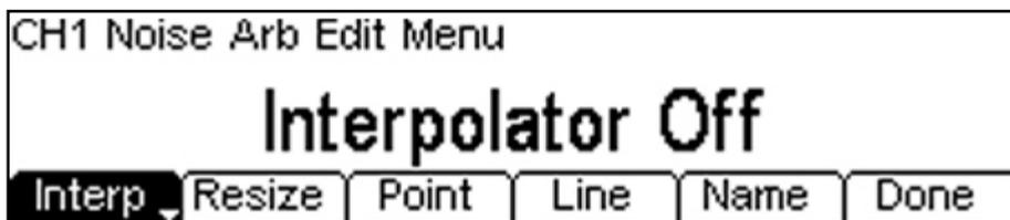
Pressing the **Interp** soft-key alternates between Interpolator Off and Interpolator On. Whatever the waveform length it will be increased to 4096 points internally when it is used. The interpolator setting defines whether this is done by repeating points or by straight line interpolation.
