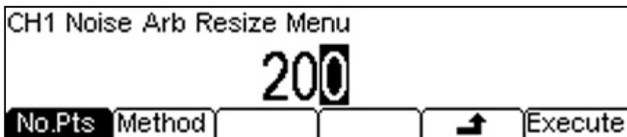
The number of points in a waveform can be within the range 1 to 2048. Default waveforms have only four points. The waveform size should be set prior to further editing because points cannot be added or removed other than by resize.
