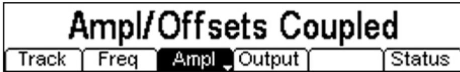
Pressing the **Ampl** soft-key alternates between Amplitude and Offsets Not Coupled and Amplitude and Offsets Coupled.
