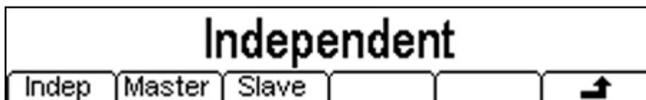
The normal mode of operation is Independent, but the generator can be combined with a second similar instrument in order to add channels.
