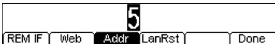
Pressing the **Addr** soft-key shows the current address setting in the edit box and allows it to be set within the range 0 to 30 using the numeric keypad or spin wheel.
