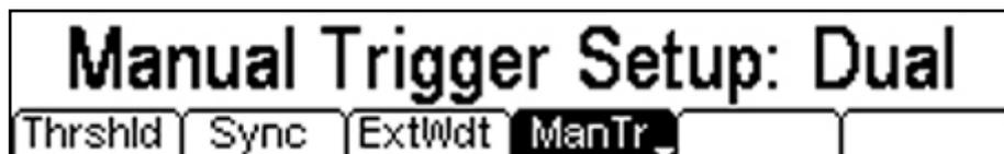
Pressing the **ManTr** soft-key alternates between Manual Trigger Setup: Single and Manual Trigger Setup: Dual.
