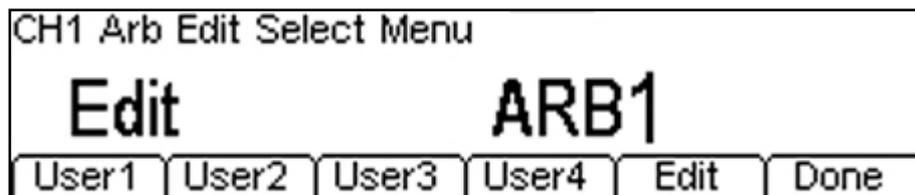
The four keys User1 thro User4 represent the four arbitrary waveforms stored within the instrument. These have default names of ARB1 thro ARB4, but these names can be changed by the user. By default each waveform is a full amplitude square wave of 4 points.
