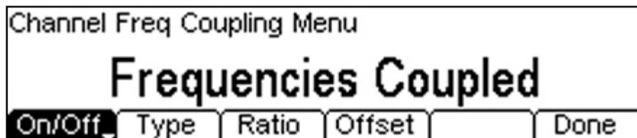
Pressing the **On/Off** soft-key alternates between Frequencies Not Coupled and Frequencies Coupled.
