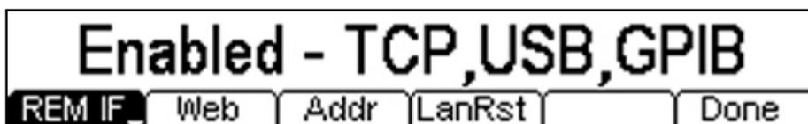
Available options are TCP (LAN) only, USB only, GPIB only, and TCP, USB and GPIB simultaneously.
