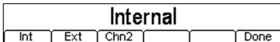
When the source is Internal, the two soft-keys on the right hand side of the modulation menu provide control of the internal modulation source.
