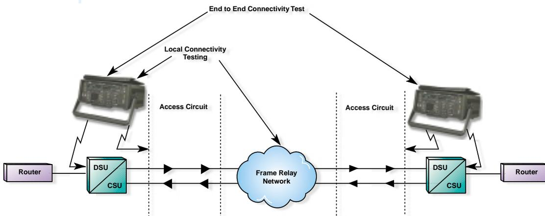
*Perform extensive frame relay testing with speeds up to 8Mb/s.*
