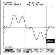
Figure 3B. Three-phase, non-linear load current waveform.
