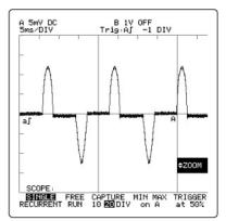
Figure 3A. Single-phase, non-linear load current waveform.
