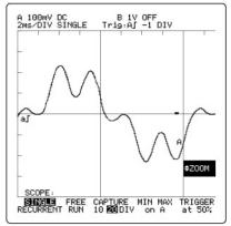
Figure 2A. Distorted current waveform.
