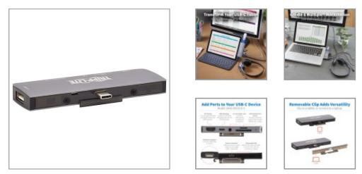
USB-C dock connects to your laptop, tablet or smartphone to add 4K HDMI, USB-A, PD Charging and memory card slots to its USB-C port.
