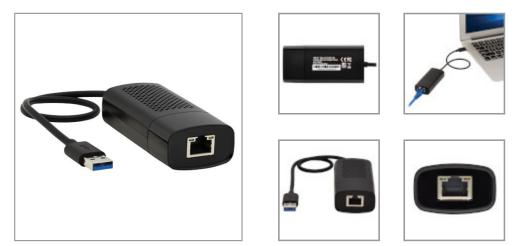
Connects the USB-A port on your laptop or PC to a wired Ethernet network at very fast 2.5 Gbps speeds with no network card needed.
