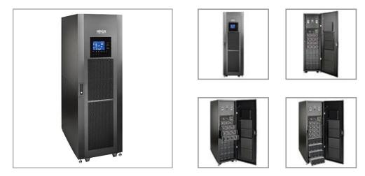
3-phase 20kVA UPS system offers network-grade power protection in a highly configurable, modular and scalable medium-chassis rack-width frame. Internal battery modules can support a full load up to 10 minutes.
