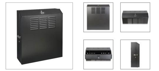
Wall-mount cabinet secures and organizes 5U of 19-inch rack equipment in network wiring closets and other locations with limited floor space. Houses equipment up to 20 inches deep, but extends less than 10 inches from wall.
