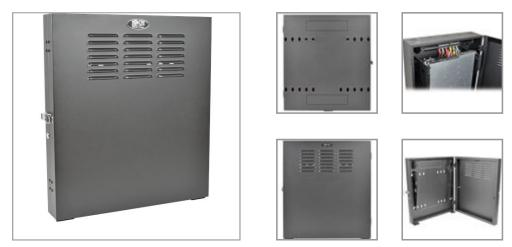
Wall-mount cabinet secures and organizes 2U of 19-inch rack equipment in network wiring closets and other locations with limited floor space. Houses equipment up to 20 inches deep, but extends less than 5 inches from wall.
