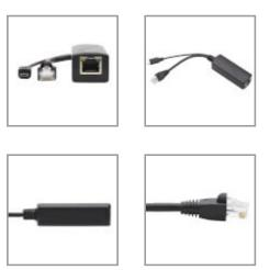
Active PoE splitter separates 5V 1A power to a USB Micro-B plug and 10/100/1000 Mbps Gigabit Ethernet data to an RJ45 plug.
