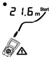
Figure 6.16 Short on Coaxial Cabling
