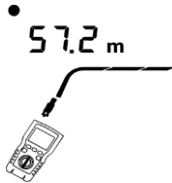
Figure 6.15 Open on Coaxial Cabling
