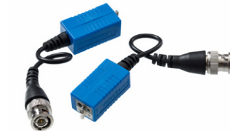
HDB-RJPT2 5MP Video Balun, CAT5 or Higher CVI 720P 400m, 1080P 250m, 4/5MP 200m TVI 720P/1080P 250m, 4/5MP 200m AHD 720P 350m, 1080P/4/5MP 200m
