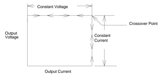
Figure 3 Constant Voltage vs. Constant Current Relation Diagram
