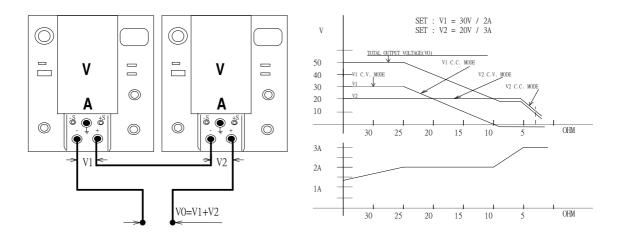
Figure 4 Serial Connection Diagram
