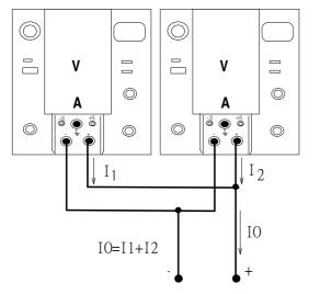
Figure 6 Parallel Connection Diagram
