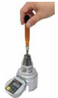
Torque checking figure for BMRD with BTGE-G
