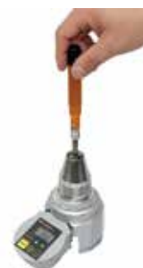
BMRD torque checking with BTGE-G.
