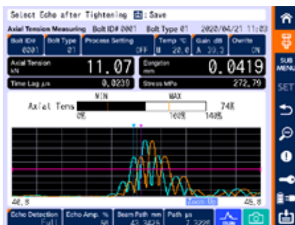
Waveform before & after giving loading
