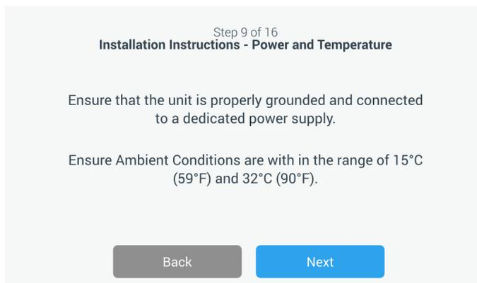
**Figure 20.** Installation Instructions (Power and Temperature) Screen
