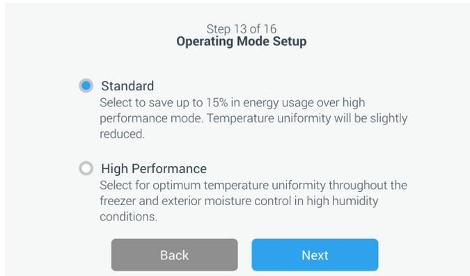
**Figure 24.** Operating Mode Setup Screen
