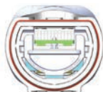
Figure 5: Battery plate unlock position
