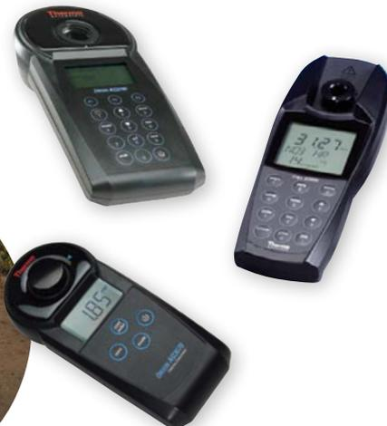
Colorimeters can be used to measure the amounts of disinfectants and their byproducts, and the concentration of various inorganic and organic chemicals. Turbidity meters help to determine the number of microorganisms in the water, or to measure cloudiness caused by flooding and run-off.
